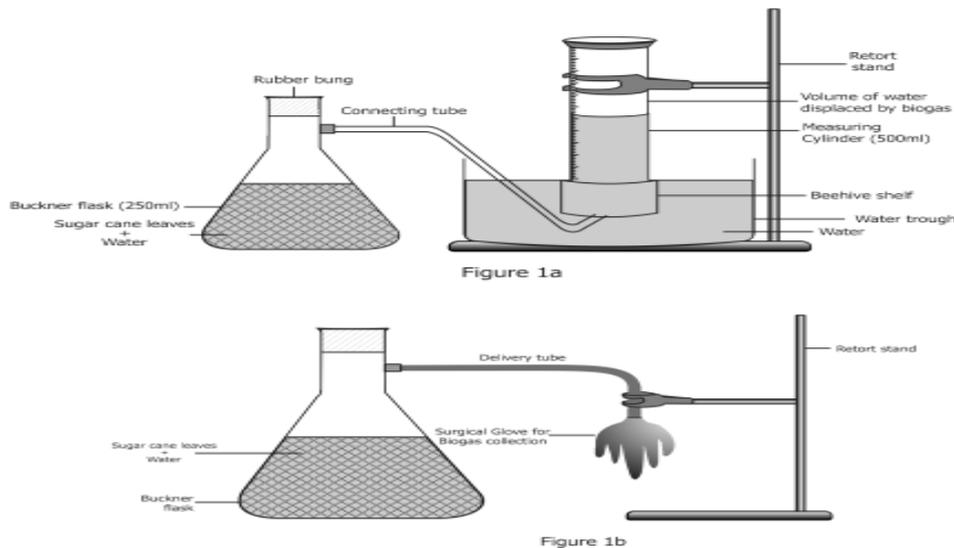
**Fig 1.** Set up for biogas production from sugar cane leaves
