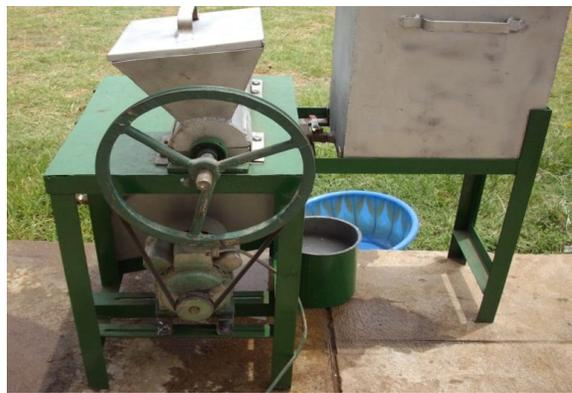
**Figure 1:** Pictorial View of the Cowpea Dehulling Machine
