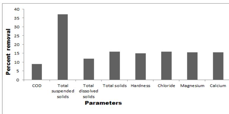
**Figure 1:** Percent removal of various pollution parameters in sawdust treated textile effluent
