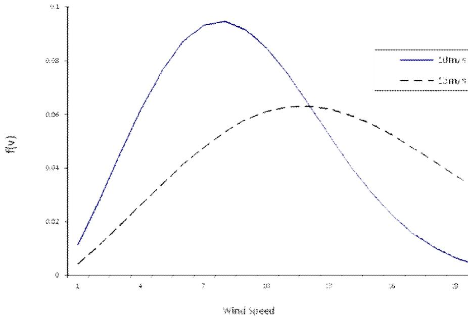
Figure.2 Weibull Wind Speed Distribution
