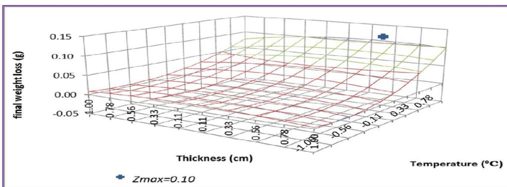
**Figure 1:** Response Surface Curves of the Effects of Temperature and Thickness of yam slices on the final weight loss of yam chips during drying
