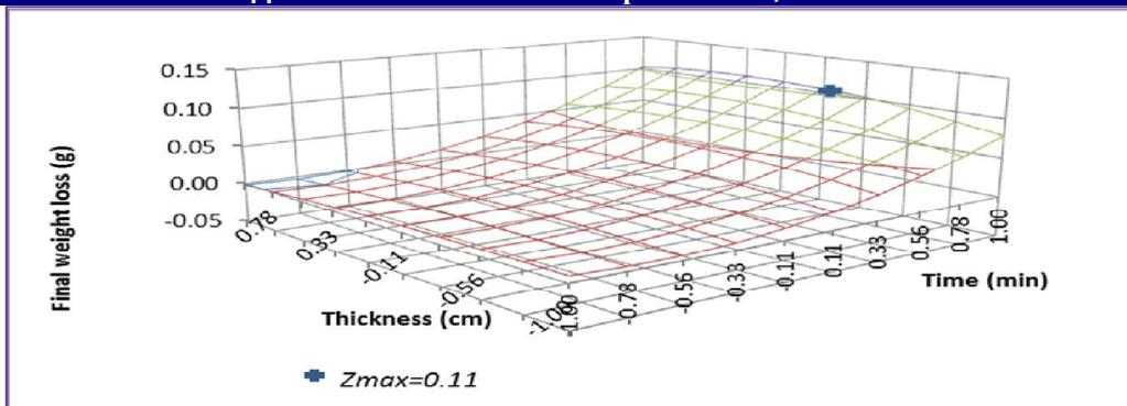
Figure 2: Response Surface Curves of the Effects of Thickness of yam slices and Time of Drying on the final weight loss of yam chips during drying
