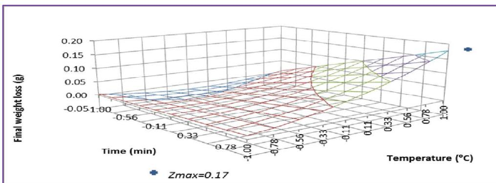
Figure 3: Response Surface Curves of the Effects of Temperature and Time of Drying on the final weight loss of yam chips during drying
