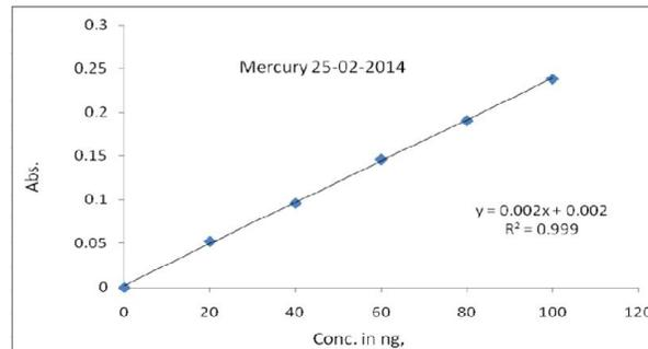
Fig 1- Calibration Curve of Mercury
