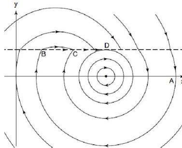
**Figure 4.** The phase portrait for a spring-mounted, rigid block on a conveyor belt.
