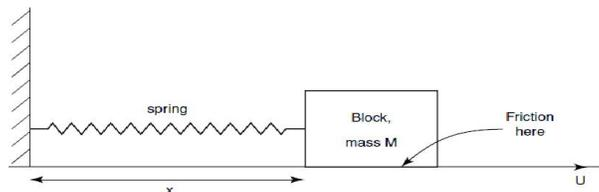
**Figure 3.** A spring-mounted, rigid block on a conveyor belt.
