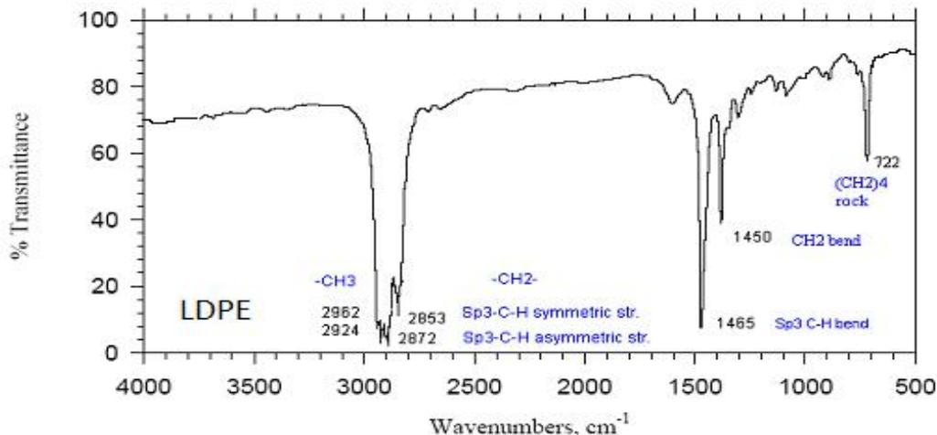
Fig 1. Infrared Spectrum of LDPE.
