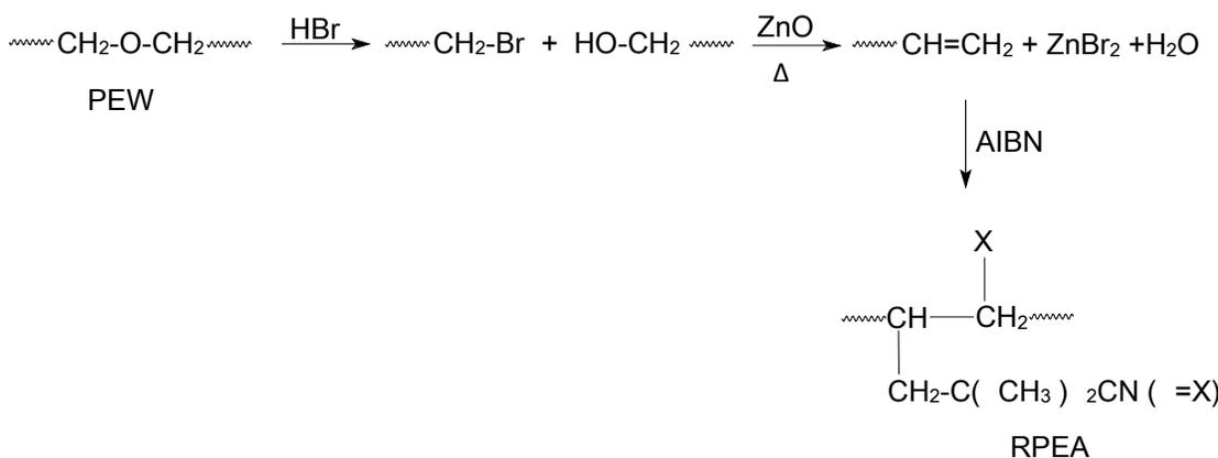
Fig 5. Chemical change during chemical treatment of waste PE.
