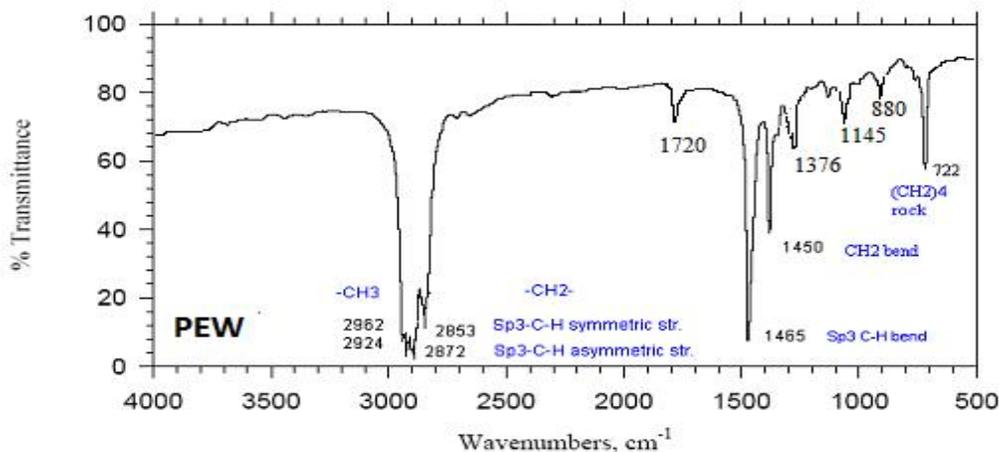
Fig 2. Infrared spectrum of polyethylene waste (PEW).
