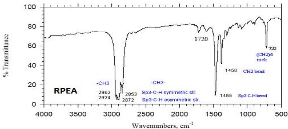
Fig 3. Infrared spectrum of RPEA.
