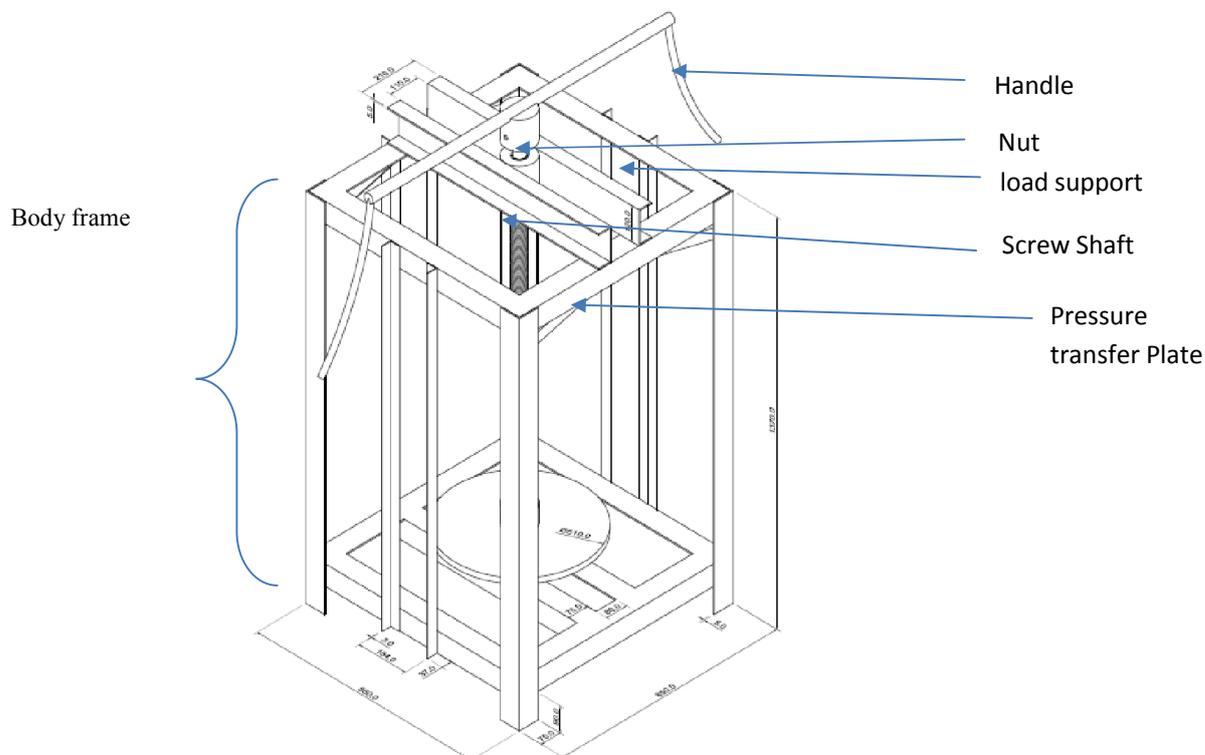
**Figure 1.** Isometric projection of single pole cassava mash dewatering press
