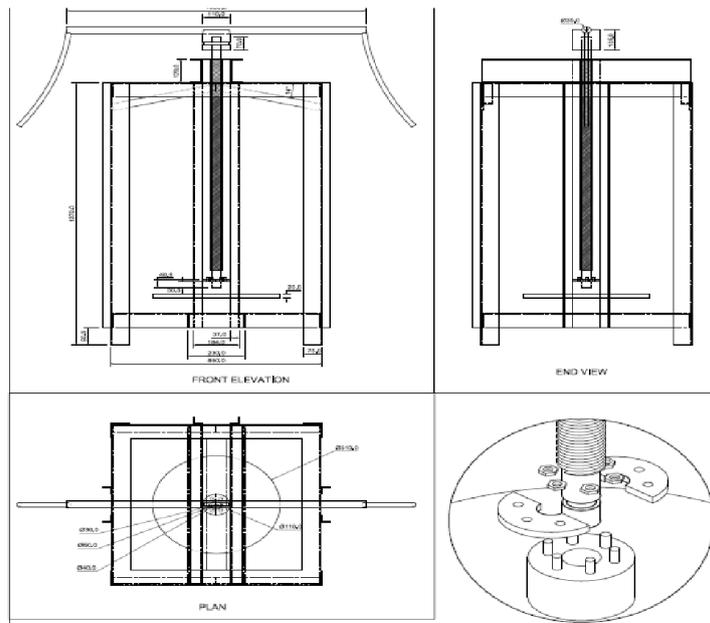
**Figure 2.** Orthographic projection of single pole
