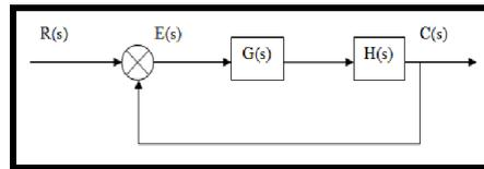
Fig 5: Closed Loop Control System (Series Connection)
