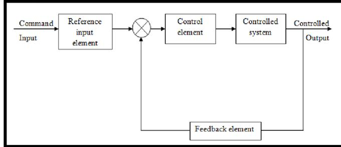
Fig 2: Closed Loop Control System
