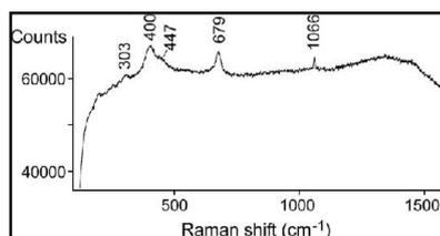
**Fig. 8.** Raman spectrum of chrysocolla in the plaster paintings.
