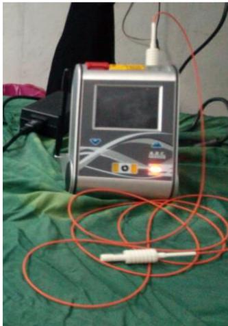
**Fig (1):** A 980 nm diode laser system
