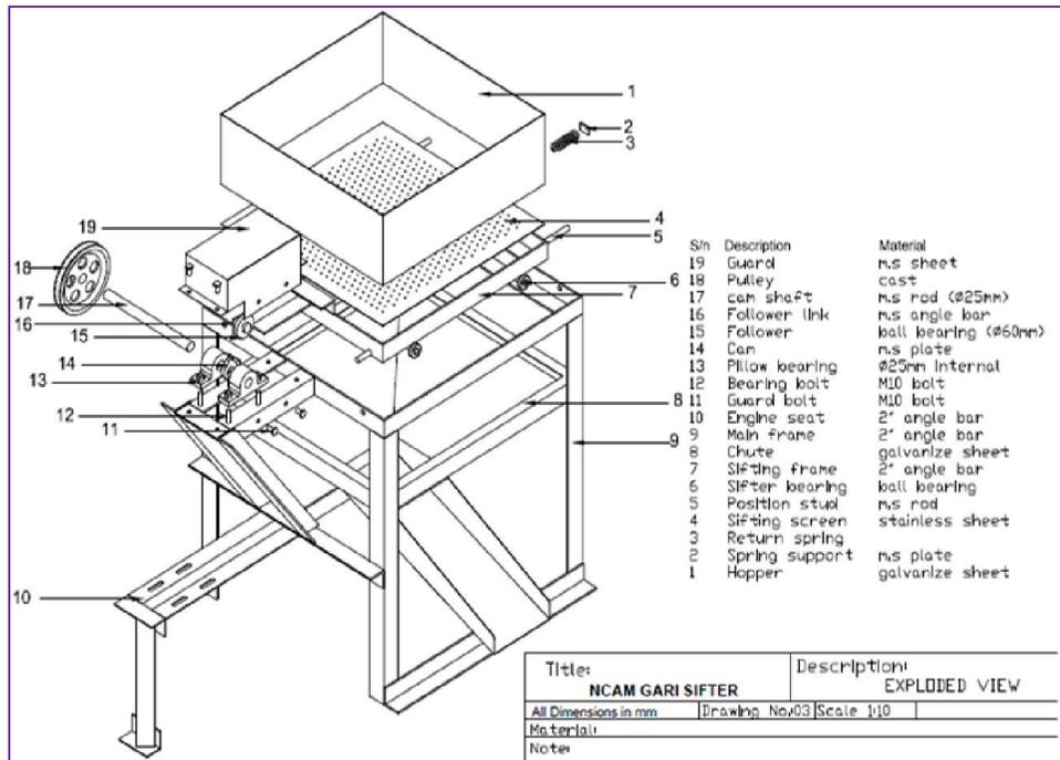
Fig. 2: Exploded view of the sifter
