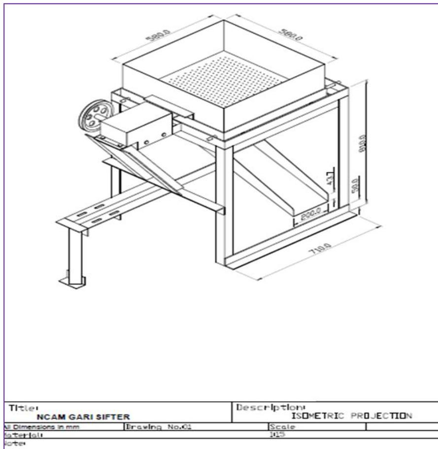
Fig 3: Isometric projection of the sifter.
