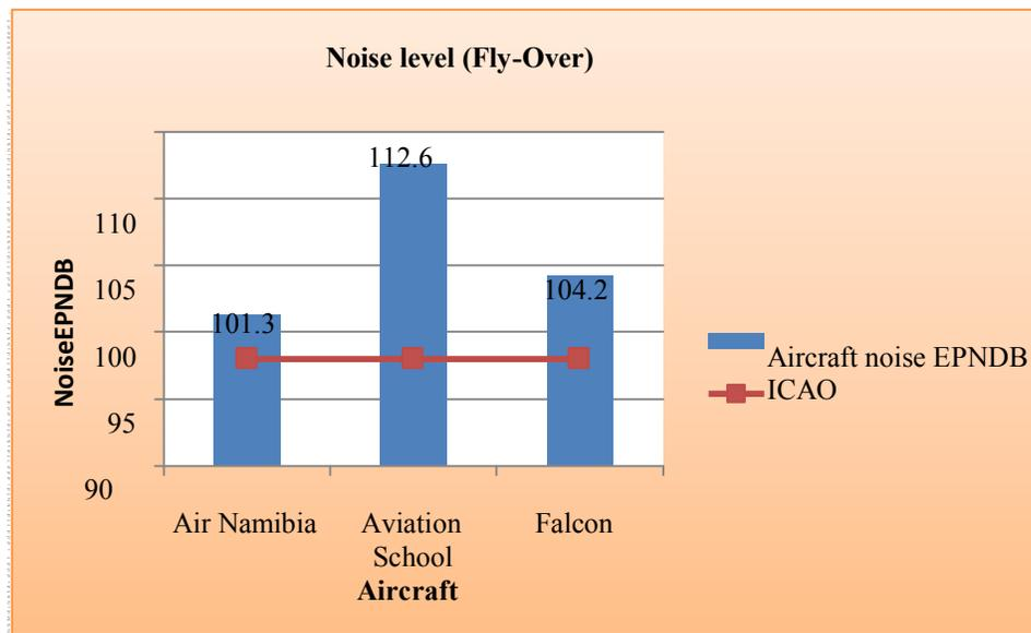
Fig 6: Fly-over noise levels vs ICAO standards
