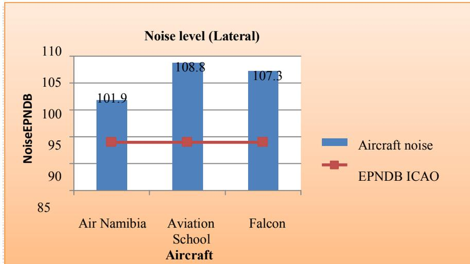
Fig 5: Lateral noise levels vs ICAO standards
