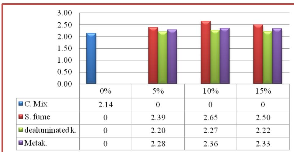
Fig 10. Elastic Modulus of Concrete Mixes ( $\times 10^5$  kg/cm<sup>2</sup>)
