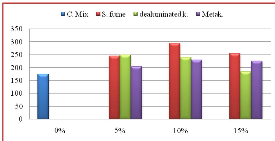
Fig 4. Compressive Strength of Concrete Mixes after 7 days
