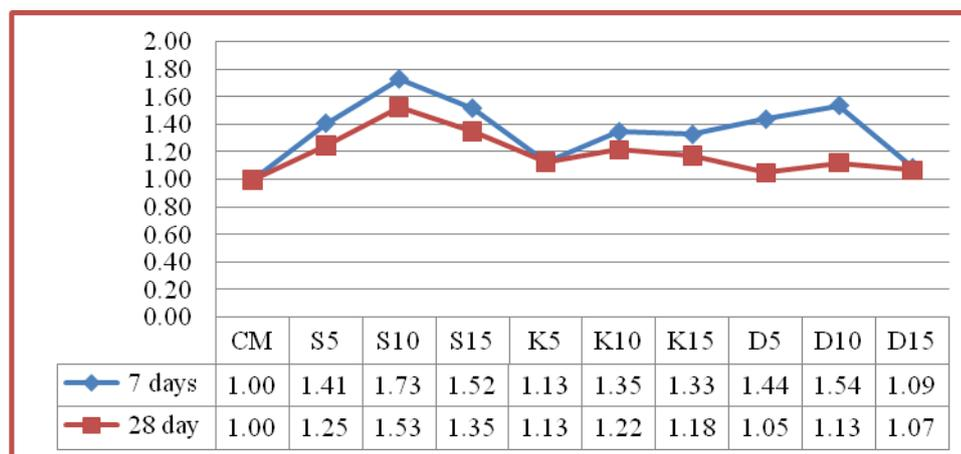
Fig 6. Relative Compressive Strength of Concrete Mixes to Control Mix
