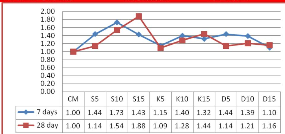
Fig 9. Tensile Strength of concrete Mixes Relative to Control Mix
