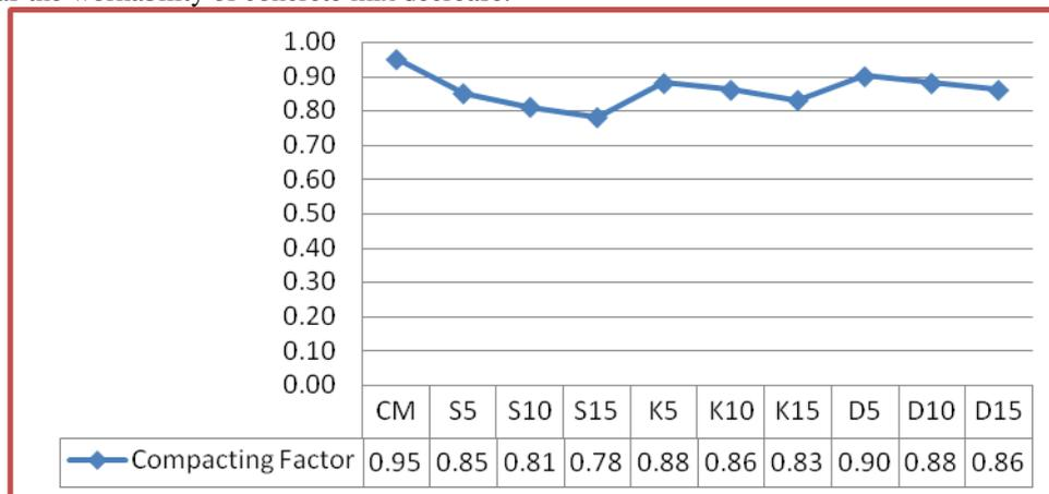
**Fig 3.** Compacting Factor (Workability) of Concrete Mixes
