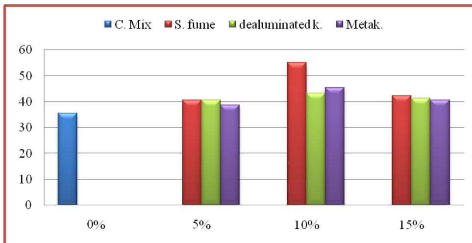
**Fig 8.** Tensile Strength of Concrete Mixes after 28 days
