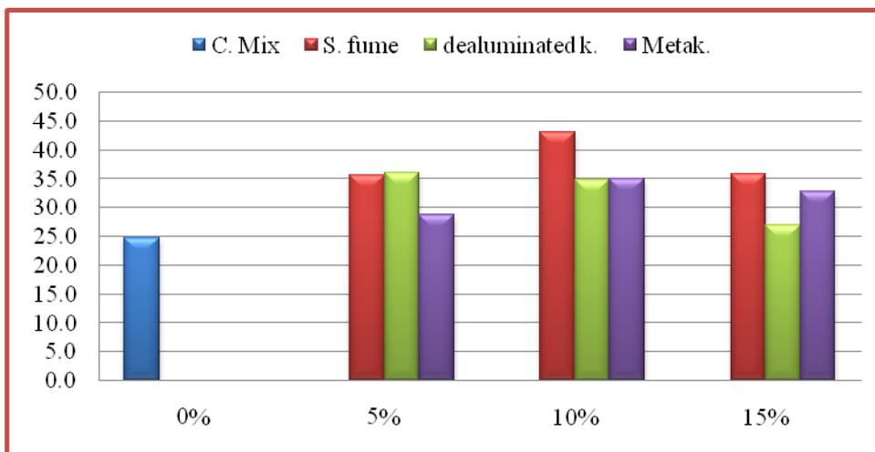
**Fig 7.**Tensile Strength of Concrete Mixes after 7 days
