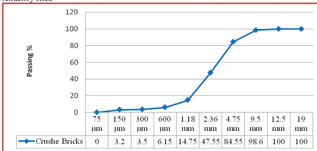
Fig 2. Grading of Aggregate
