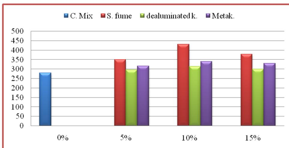
Fig 5. Compressive Strength of Concrete Mixes after 28 days
