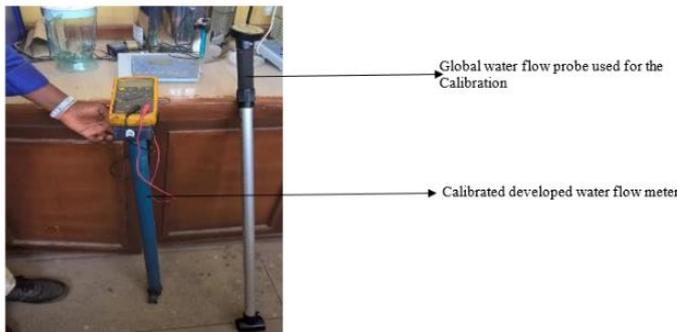
Figure 3.2: Pictorial view of the locally developed water flow meter and the standard used the calibration
