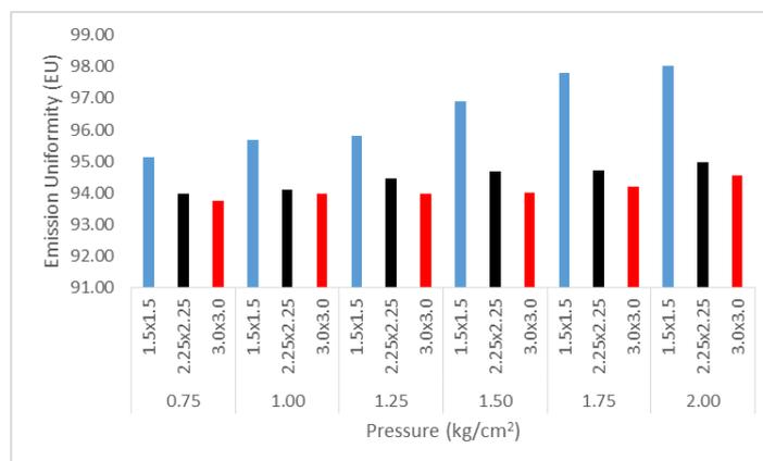
**Fig 5:** Emission uniformity for micro-irrigation sprinkler system
