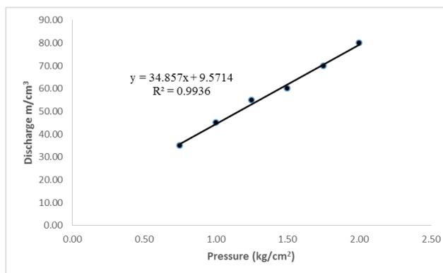
**Fig 2:** Pressure-Discharge relationship for micro-irrigation sprinkler system
