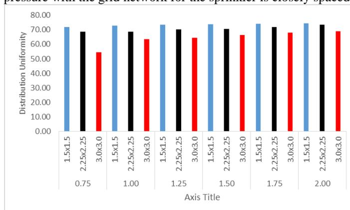
**Fig 6:** Distribution Uniformity for micro-irrigation sprinkler system
