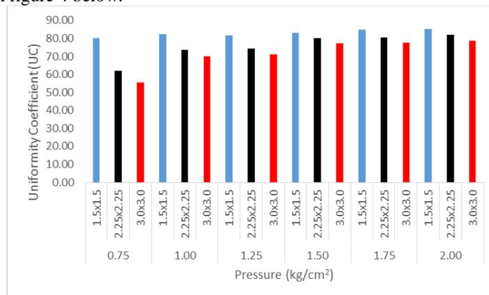
**Fig 4:** Uniformity coefficient for micro-irrigation sprinkler system.
