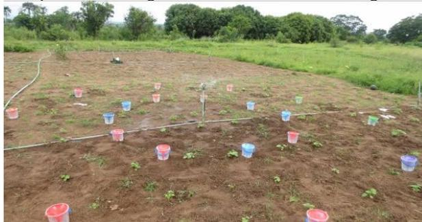
**Fig 1:** Micro-irrigation sprinkler system showing water cans in grids.
