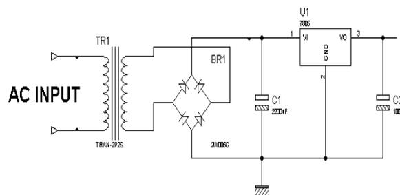
Fig. 2 Circuit diagram of the regulated power supply
