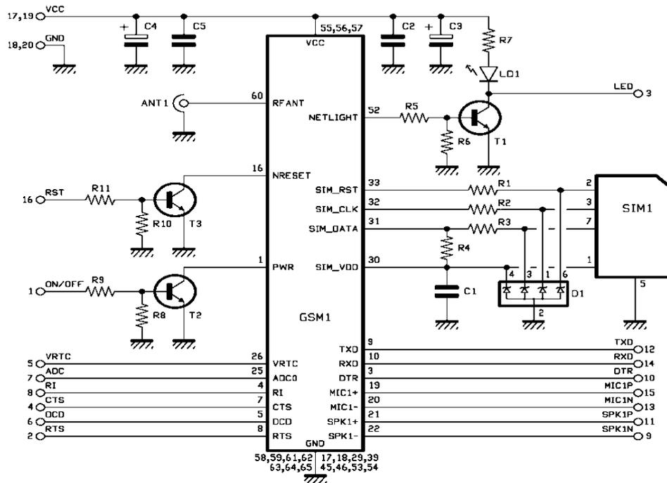
Fig. 3: Circuit diagram of SIM900 (GSM module)
