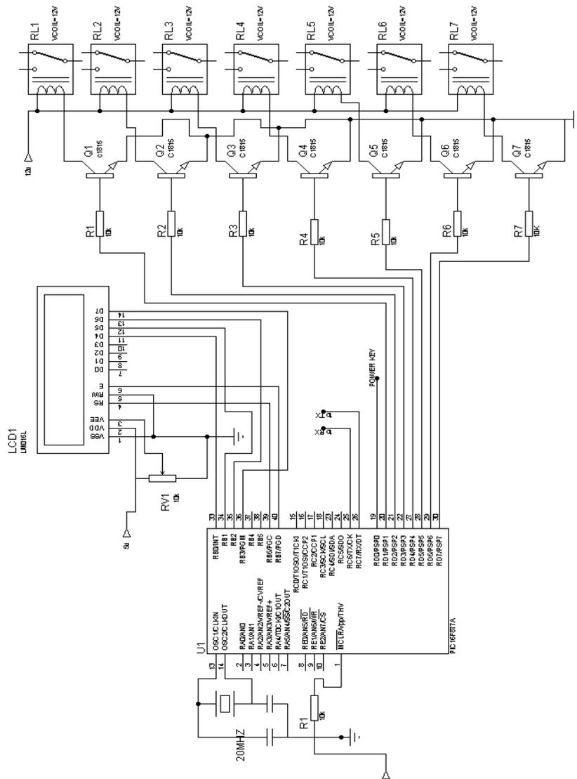
Fig.5: Circuit diagram of the GSM Based Home Devices control system
