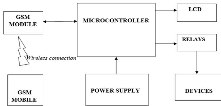
Fig.1 Block diagram of the GSM based home devices control system
