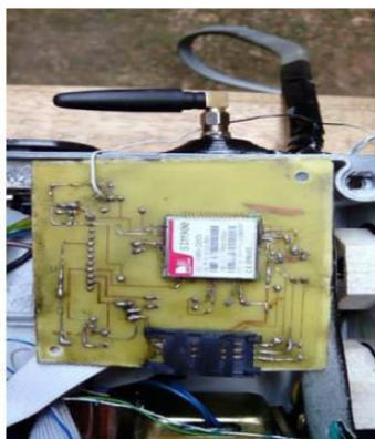
Fig 6: GSM module
