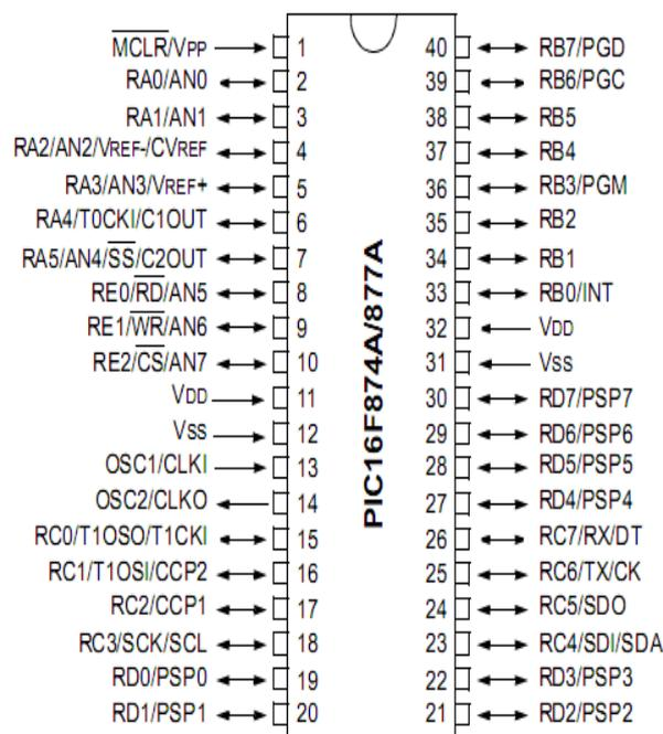
Fig. 4: The pin diagram of PIC16f877A (Microcontroller)
