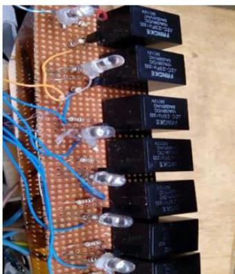
Fig 7: The relay, relay driver and indicator module
