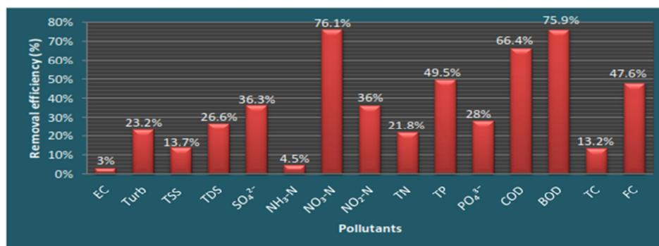
**Fig 1:** Pollutants removal performance of BTGH Anaerobic Baffled Reactors.
