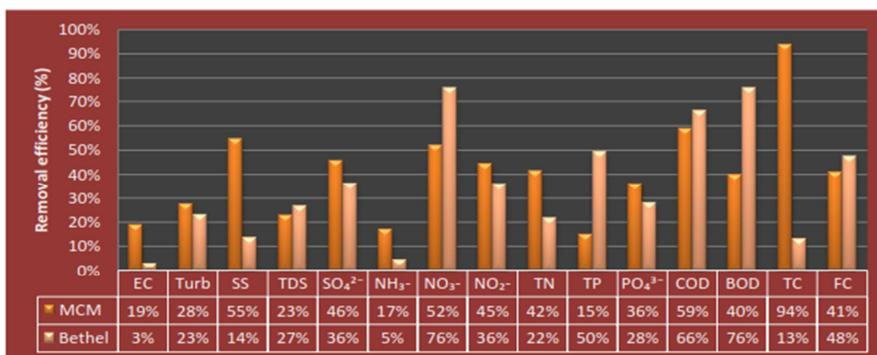
Fig 4: Comparisons of the removal efficiency (%) of the hospitals WWTPs
