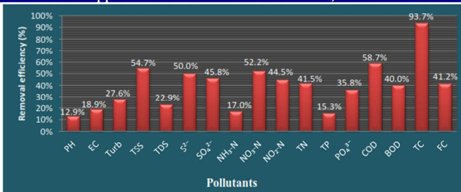
Fig 3: Pollutants removal performance of MCM Anaerobic Digesters.
