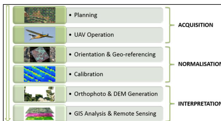
Fig 1: Flowchart adopted for 3D mapping using Drone Technology
