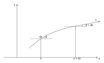
Let  $\lambda_0$  be the uniform linear density of rest mass of the string. Then neglecting the effect of gravitation then, the vertical force acting at the end of the element at x is given by  $T\sin\theta$ . Also the vertical force acting at the end of the string at x+dx is giving by  $T\sin(\theta + d\theta)$ . consequently, the net vertical force acting on the element of the string, F, is given by;
