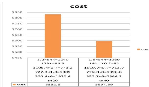
**Fig 1.** Cost comparison of externally and internally cured concrete per cu.m.
