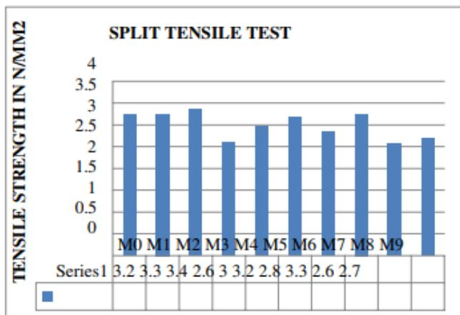
**Fig 4:** Graph shows 28 days of split tensile strength for normal concrete and concrete made with fly ash and GGBS as partial replacement of cement
