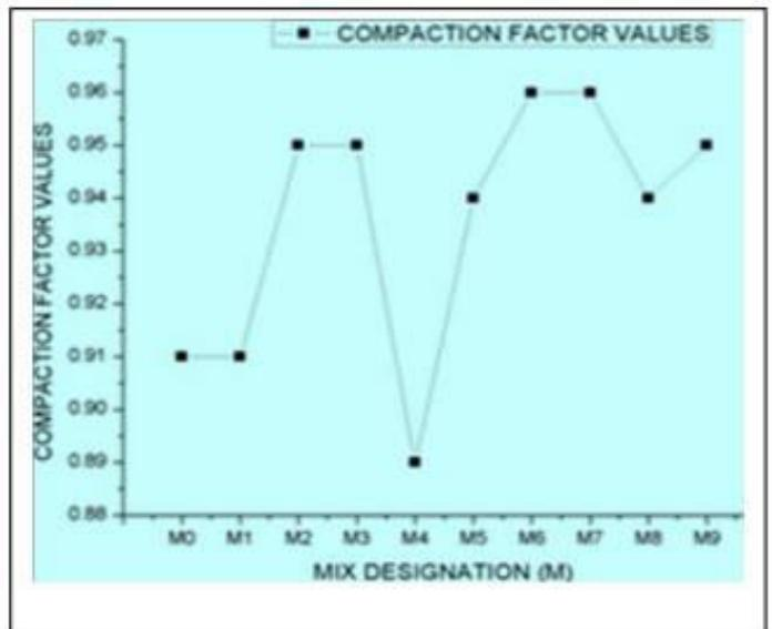
Fig 2: Graph shows compaction factor values for normal concrete and concrete made with fly ash and GGBS as partial replacement of cement
