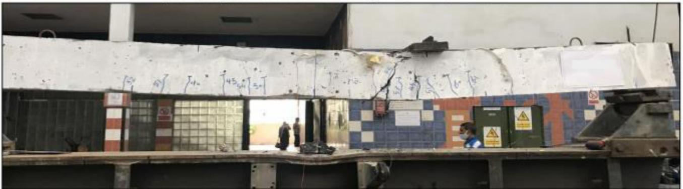
**Fig.6 crack pattern and the failure in specimen 120UH25-1%**
