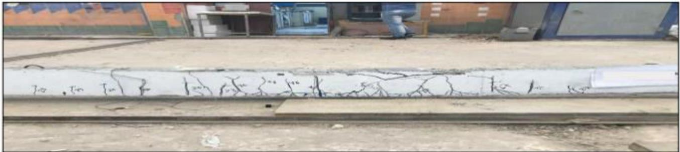
**Fig.2** Crack pattern and the failure in specimen 60WF25-1%
