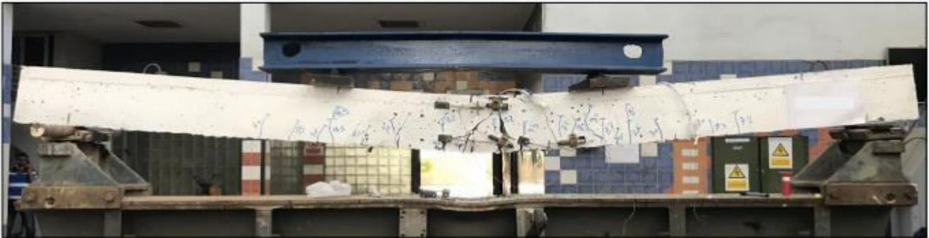
**Fig.5 crack pattern and the failure in specimen 120UH25-0.7%**
