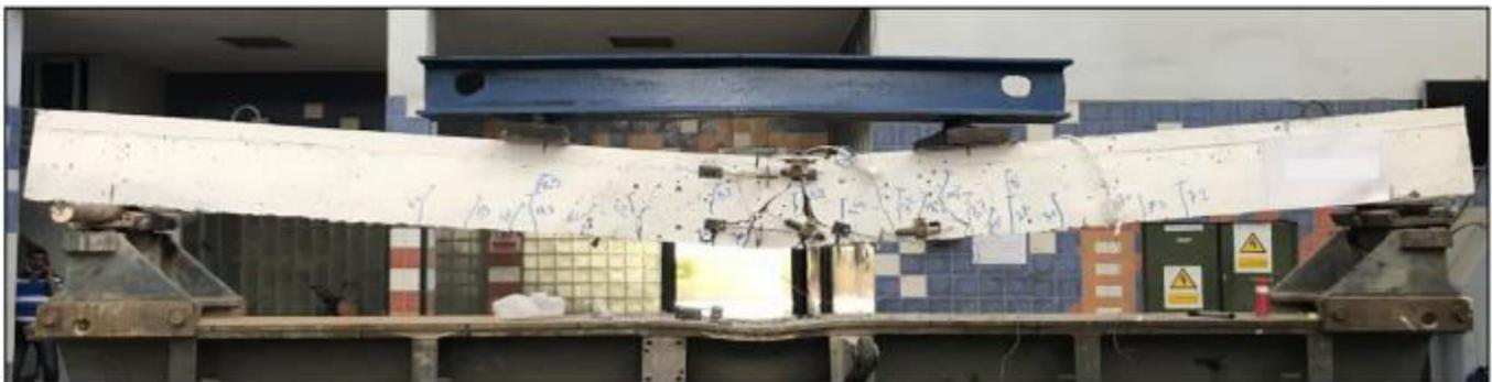
**Fig.7 crack pattern and the failure in specimen 120UH25-1.4%**
