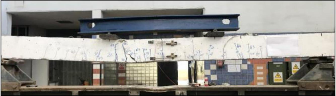
**Fig.4 crack pattern and the failure in specimen 80BF25-1%**
