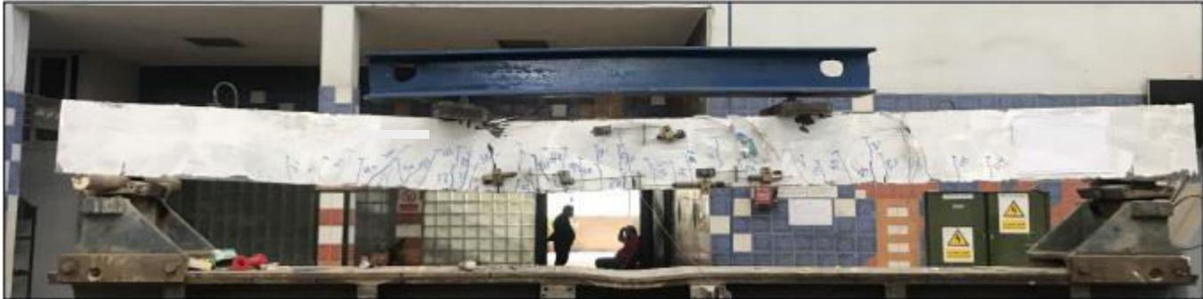
Fig.9 crack pattern and the failure in specimen 120UH25-2.2%
