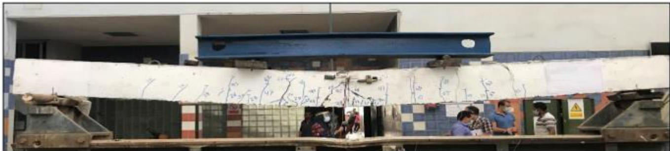
**Fig.3** Crack pattern and the failure in specimen 60BF25-1%
