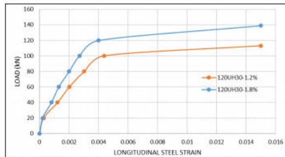
Fig.27 Load –longitudinal steel strain Curve for Group I D/W=3
