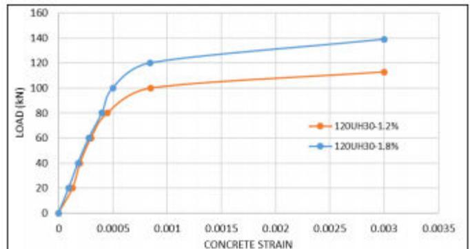
Fig.22 Load –Concrete strain Curve for Group I D/W=3
