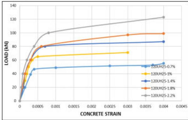
Fig.23 Load –Concrete strain Curve for Group.II
