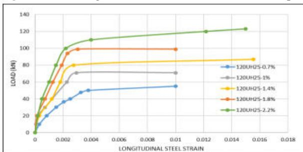
Fig.28 Load – Longitudinal Steel Strain Curve for Group.II
