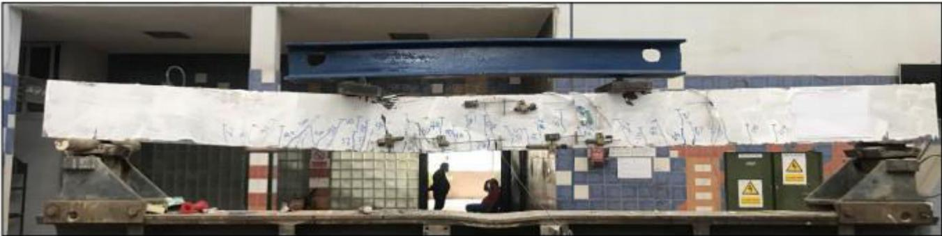
Fig.10 crack pattern and the failure in specimen 120UH25-2.2%
