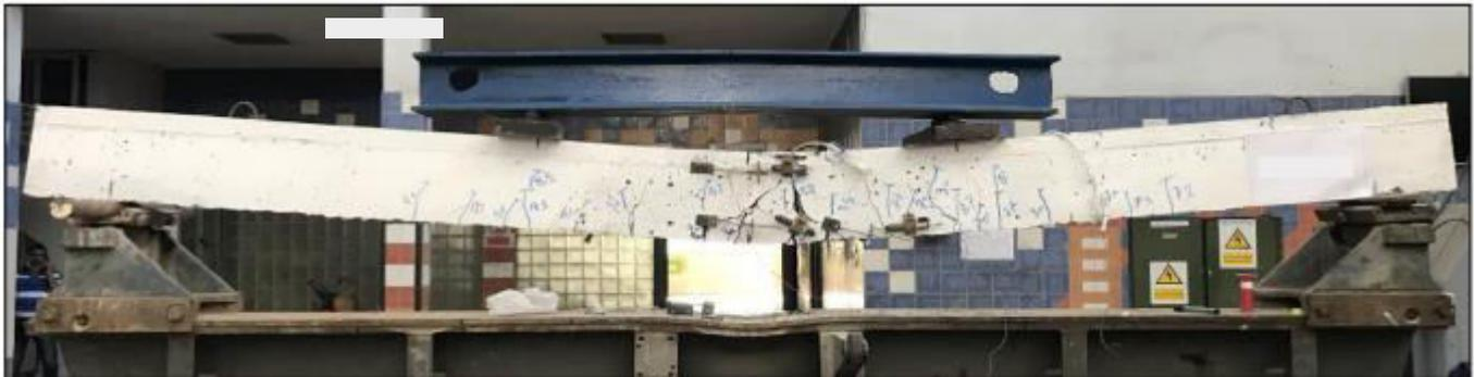
**Fig.6** crack pattern and the failure in specimen 120UH25-0.7%
