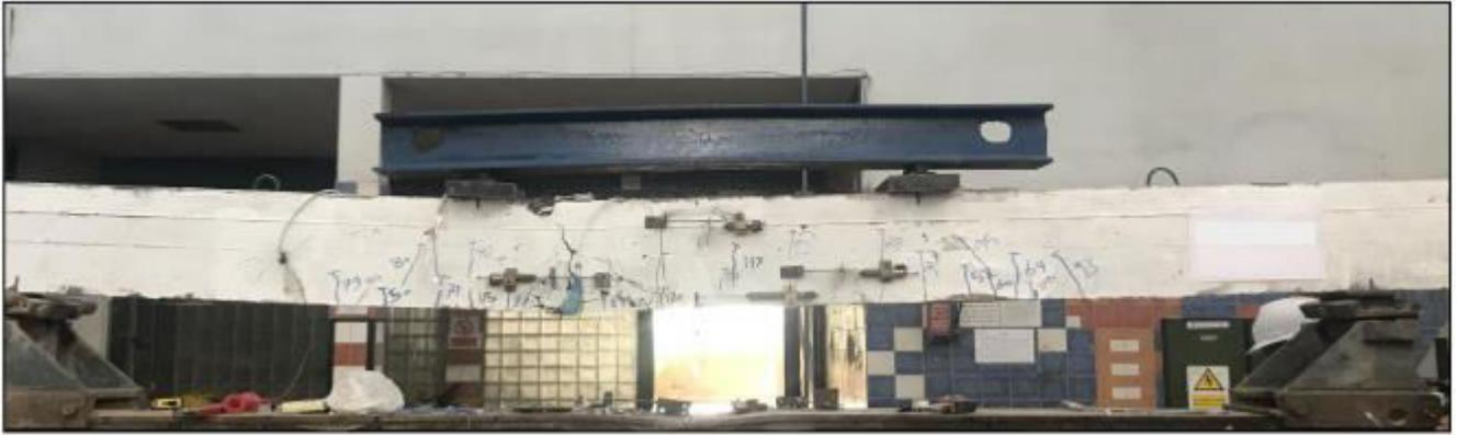
**Fig.5** crack pattern and the failure in specimen 120UH30-1.8%
