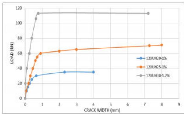
Fig.14 Effect the same reinforcement steel ratio with others cross section on load-crack width curve
