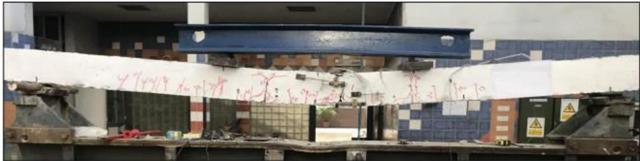
Fig.2 crack pattern and the failure in specimen 120UH20-1%
