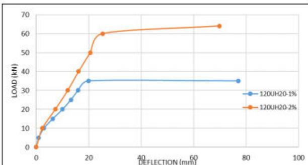
Fig.16 Load –Deflection Curve for Group I D/W=2
