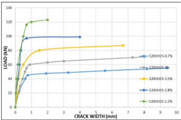
Fig.13 Load –Crack Width Curve for Group.II
