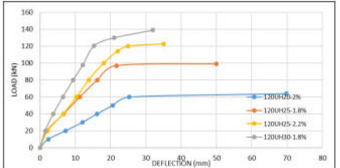
Fig.20 Effect the same double reinforcement steel ratio with others cross section on load-deflection curve
