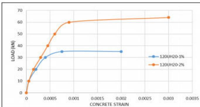
Fig.21 Load –concrete strain Curve for Group I D/W=2
