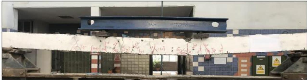
Fig.3 crack pattern and the failure in specimen 120UH20-2%
