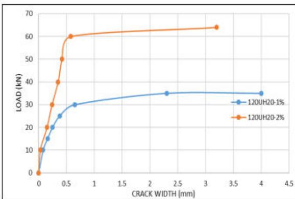
Fig.11 Load –Crack width Curve for Group I D/W=2
