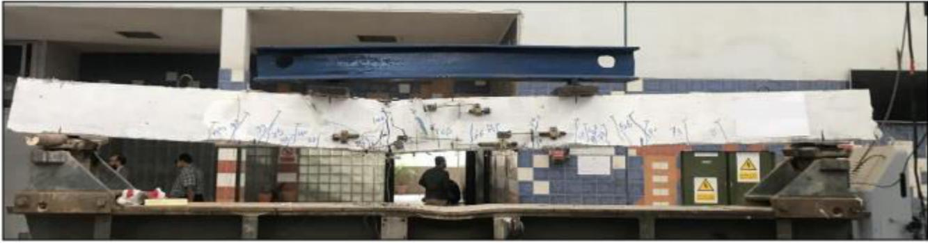
Fig.9 crack pattern and the failure in specimen 120UH25-1.8%
