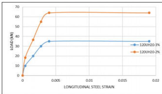
Fig.26 Load – longitudinal steel strain Curve for Group I D/W=2
