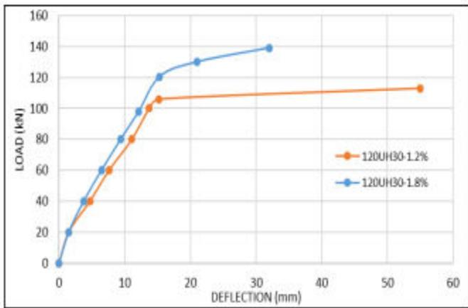
Fig.17 Load –Deflection Curve for Group I D/W=3
