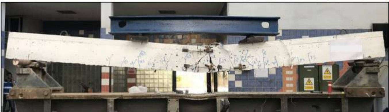
**Fig.8** crack pattern and the failure in specimen 120UH25-1.4%
