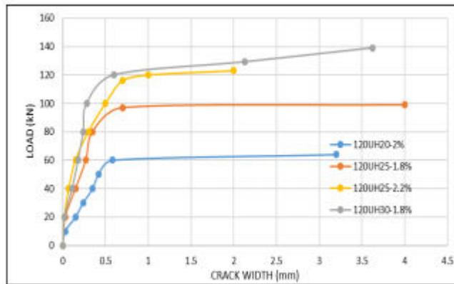
Fig.15 Effect the same double reinforcement steel ratio with others cross section on load crack width curve
