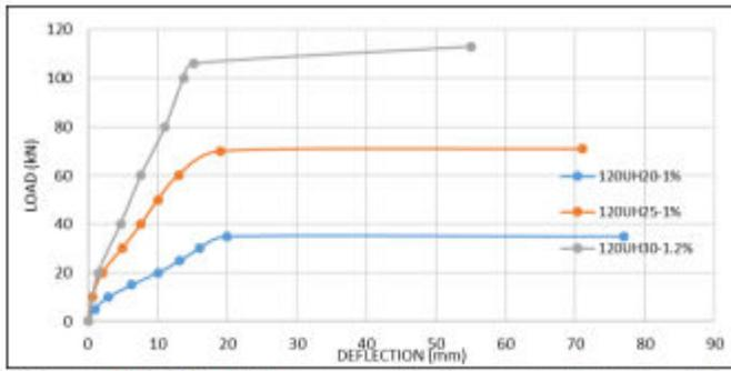
Fig.19 Effect the same reinforcement steel ratio with others cross section on load-deflection curve
