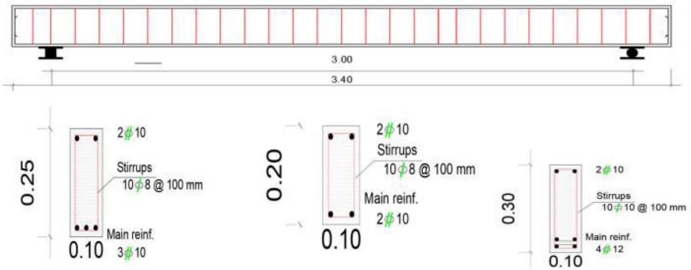
**Fig. 1** Details of specimens
