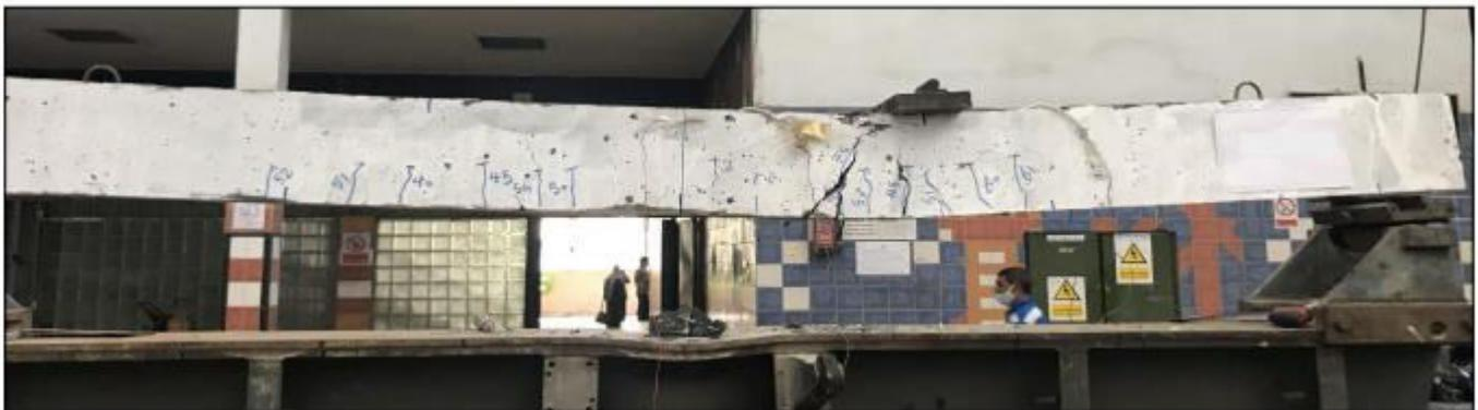
**Fig.7** crack pattern and the failure in specimen 120UH25-1%
