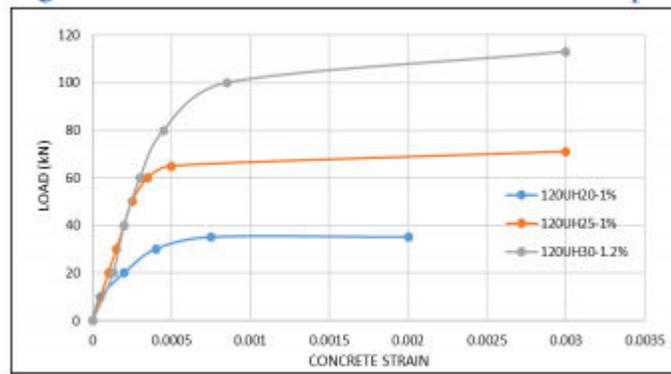
Fig.24 Effect the same reinforcement steel ratio with others cross section on load-deflection curve
