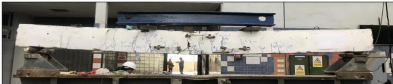
Fig.4 crack pattern and the failure in specimen 120UH30-1.2%
