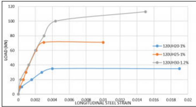
**Fig.29** Effect the same reinforcement steel ratio with others cross section on load-deflection curve
