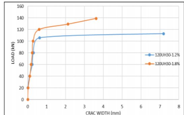
Fig.12 Load –Crack width Curve for Group I D/W=3
