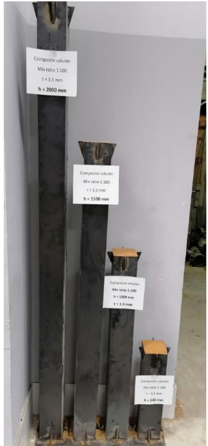
Fig 3. Specimens of Composite Columns
