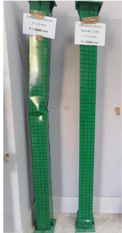
Fig 8. Failure mode of Section h/b = 16
