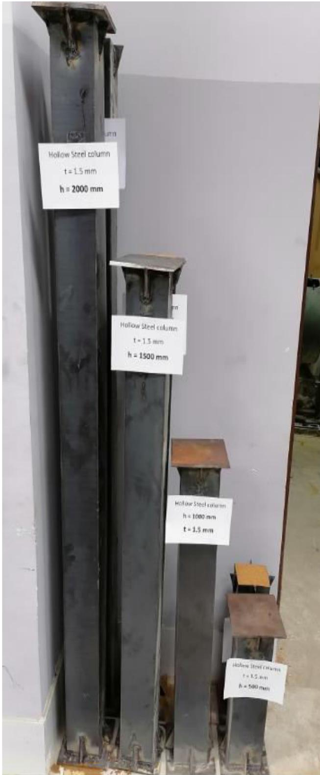
Fig 2. Specimens of Hollow Steel Columns
