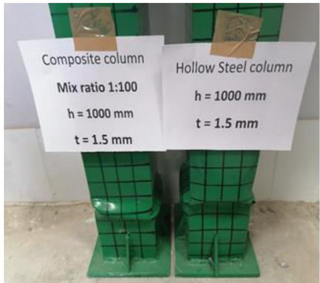
Fig 6. Failure mode of section  $h/b = 8$
