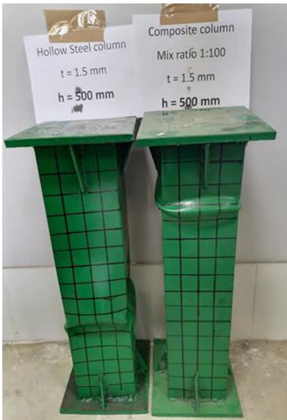
Fig 5. Failure mode of section  $h/b = 4$
