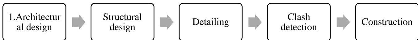
Fig 2. The steel structure processes
