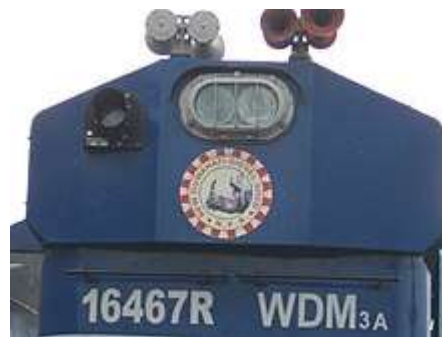
Fig. 1 Close-up of a locomotive with the classification and number; WDM3A indicates a Broad gauge (W), Diesel (D), Mixed use (M), 3100 HP (3A) locomotive
