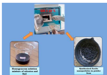
Fig. 1 Synthesis of Polyaniline/ \text{Co}_x\text{Cr}_{0.5-x}\text{Fe}_2\text{O}_4 Nanocomposites
