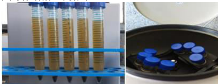
Fig 5: Centrifuge tube are placed in centrifuge machine and sample is collected in centrifuge tube
